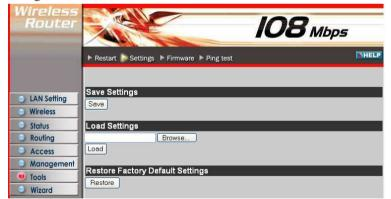
**Save Settings:** Click "Save" to save the current configuration as a profile that can load when necessary.
